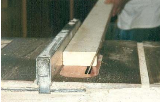
Sawing the beveled overhang (22 1/2 deg)
